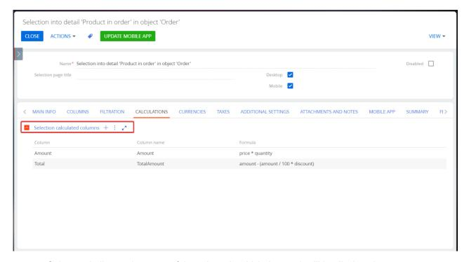
Column – indicates the name of the column in which the result will be displayed;
